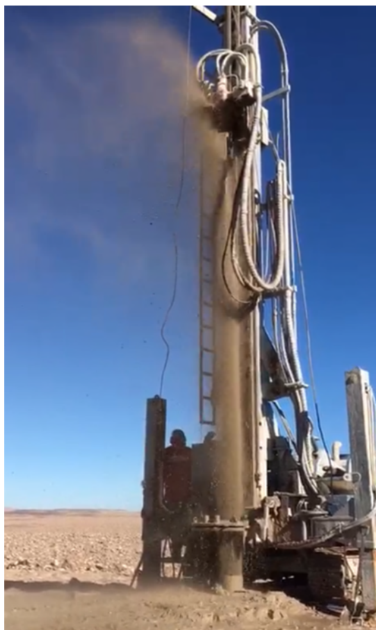
Figure 7: High pressure brine encountered in drilling
