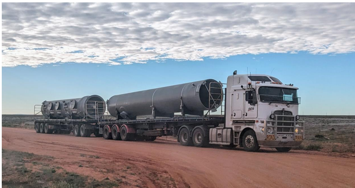
Image 1: First NIMCIX elution column entering Honeymoon uranium mine site
