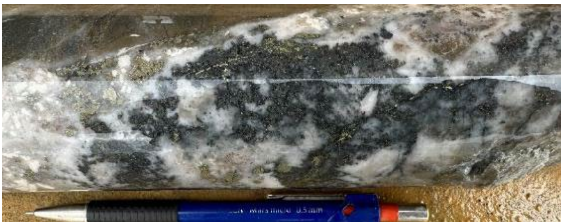
Large quartz+tennantite+chalcopyrite+pyrite vein. 543.7m. pXRF showed Fe, Cu, Zn and As>>Sb.
