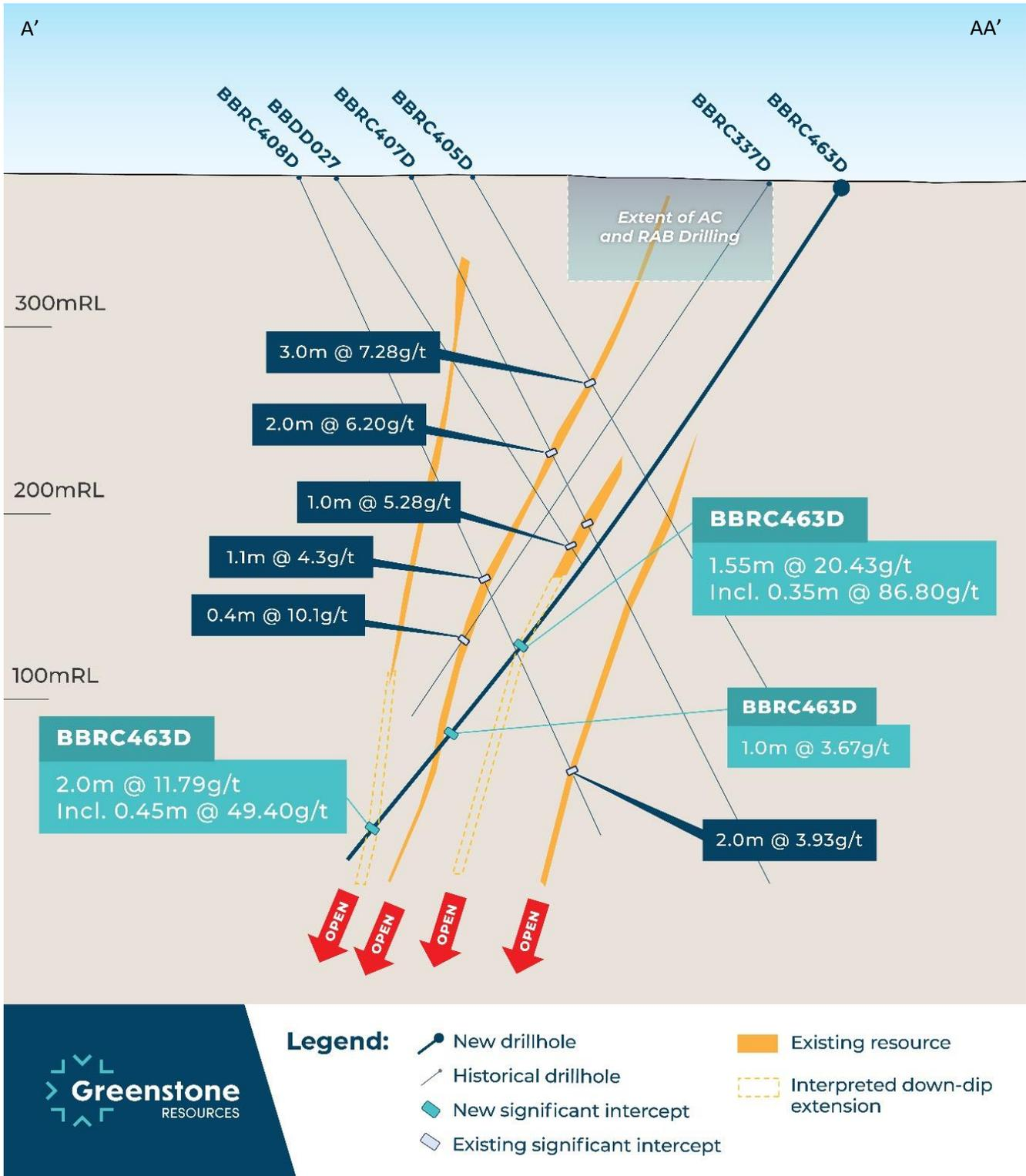
Figure 1: Cross section of BBRC463D showing current Burbanks North MRE lodes, latest reported intercepts, and interpreted down-dip extensions of mineralisation.
