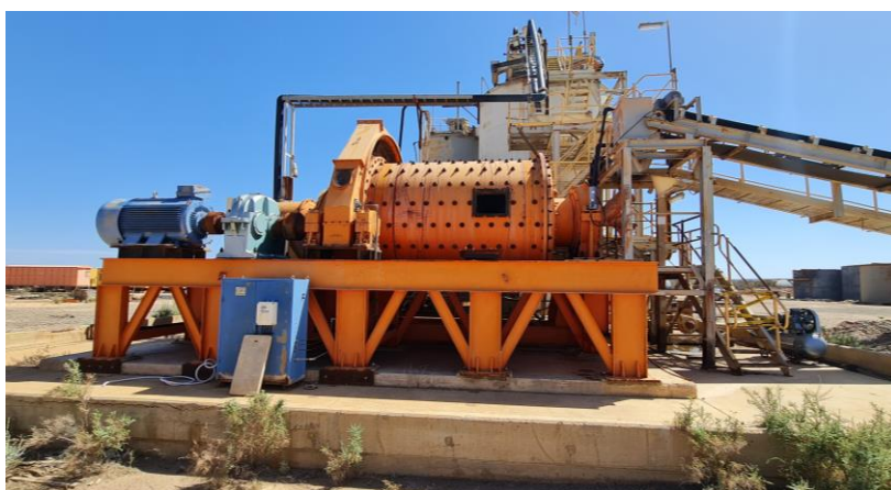
Left: Gravity Circuit. Right: 450kW Ball Mill
