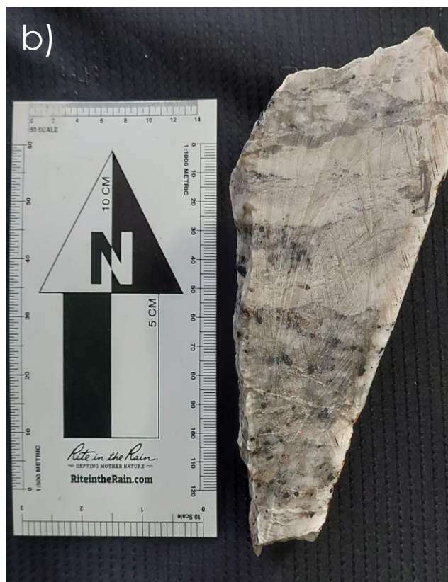
Figure 6b): G2 channel sample J083916 (2.22% Li 2 O) visually representative portion of 1m sample of leucocratic pegmatite comprising alternating bands of crystalline quartz blue-grey to white in colour (40%) and aphanitic white bands of spodumene and plagioclase (20% and 25% respectively). 3-5% black coarse (0.5 – 1cm) subhedral tourmaline and tantalite are disseminated within the quartz banding. 1-3% fine grained pale green micas (0.1 – 0.2cm) are disseminated throughout the rock. Pink to red garnet are present in trace disseminations of highly variable grain size ranging from 0.1 – 1cm.
