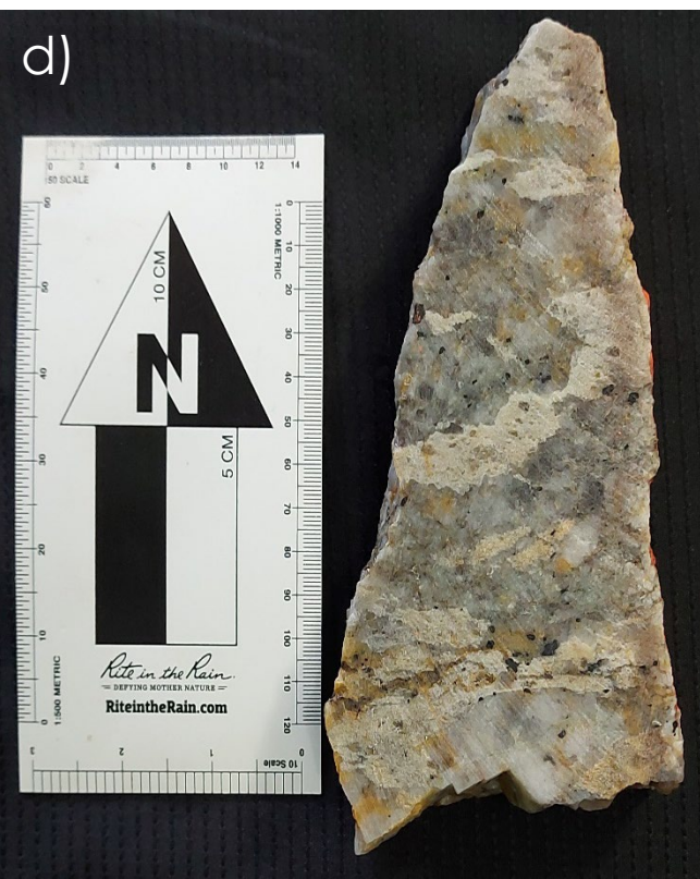
Figure 6d): G0 Channel sample J083874 2.31% \text{Li}_2\text{O} visually representative portion of 1 metre sample of leucocratic pegmatite comprising alternating bands of crystalline quartz blue-grey to white in colour (40%) and aphanitic yellowish-white bands of spodumene and plagioclase (15% and 25% respectively). White prismatic spodumene crystals range from 1 – 5 cm. 3-5% medium grained (0.1 – 0.5 cm) subhedral tourmaline and tantalite \pm columbite are dark black in colour and disseminated within the quartz banding. 5-10% fine grained pale green mica (0.1 – 0.2 cm) are disseminated throughout the rock. Pink to red garnet are present in trace disseminations of highly variable grain size ranging from 0.1 – 1 cm.
