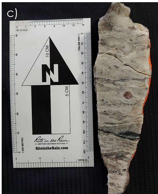
Figure 6c): G1 Channel sample J083861 2.09% \text{Li}_2\text{O} visually representative portion of 1 metre sample of leucocratic pegmatite comprising alternating bands of crystalline quartz blue-grey to white in colour (40%) and aphanitic white bands to coarse crystals of spodumene and plagioclase (15% and 25% respectively). White prismatic spodumene crystals range from 1 – 2 cm. Medium grained (0.1 – 0.5 cm) subhedral tourmaline and tantalite \pm columbite are dark black in colour and disseminated, varying between 3 – 5% within the quartz banding. 1-3% fine grained pale green mica (0.1 – 0.2 cm) are disseminated throughout the rock. Pink to red garnet present in trace disseminations of highly variable grain size ranging from 0.1 – 1 cm.
