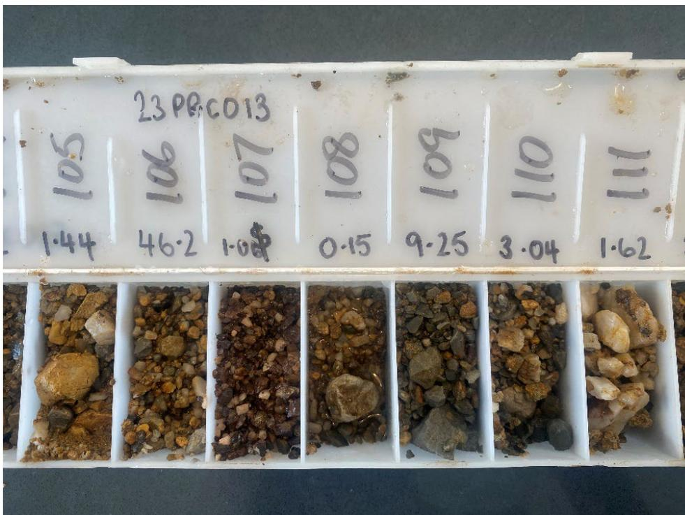
Figure 3: Drill chips from 23PRC013 with gold grades (g/t) noted above
