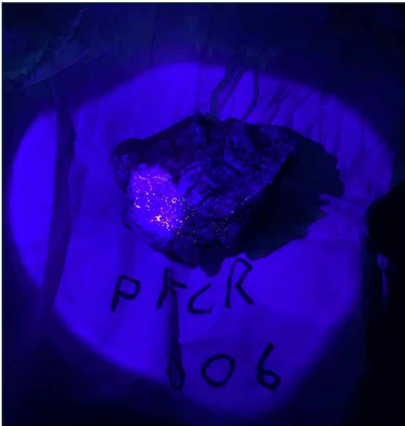
Figure 2: Rock chip sample displaying distinctive ultra-violet fluorescence 2 of potential lithium bearing minerals.
