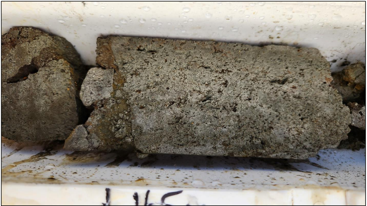
MLJDD018_164.5m_Massive pyrite in Breccia
