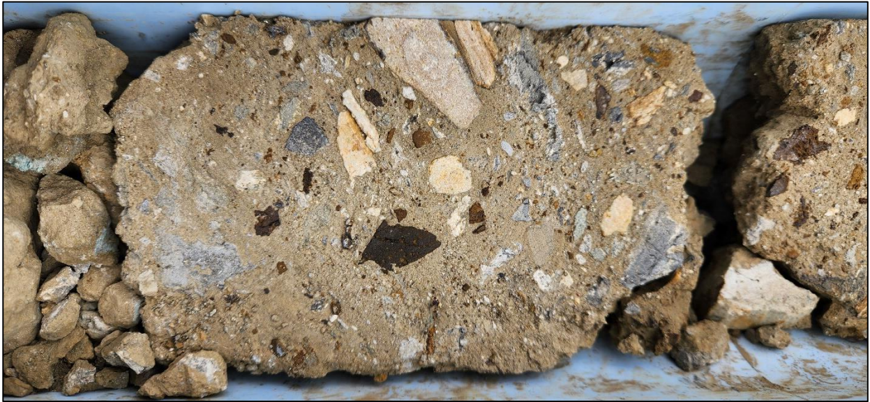
MLJDD020_178.0m_Polymictic Breccia with silica-pyrite clast
