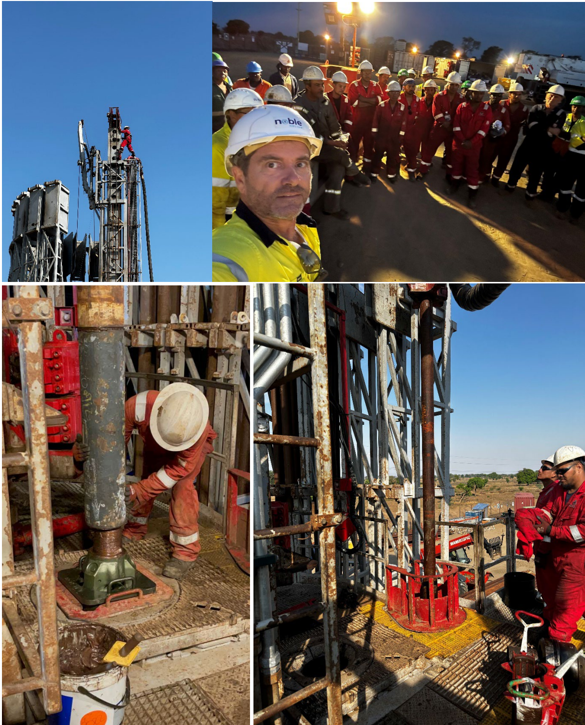
Clockwise from top left: Last-minute checks of the crown block; Pre-spud meeting with the full drilling team; Setting up drill string in the mouse hole; Attaching the first drill bit to the Mbelele-1 BHA (Bottom Hole Assembly), in preparation for spud.
