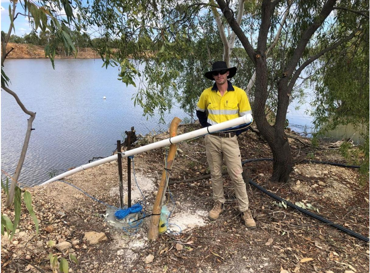
**Figure 33: Installing 'Level Logger' water depth measuring equipment at Yandan Main Pit.**
