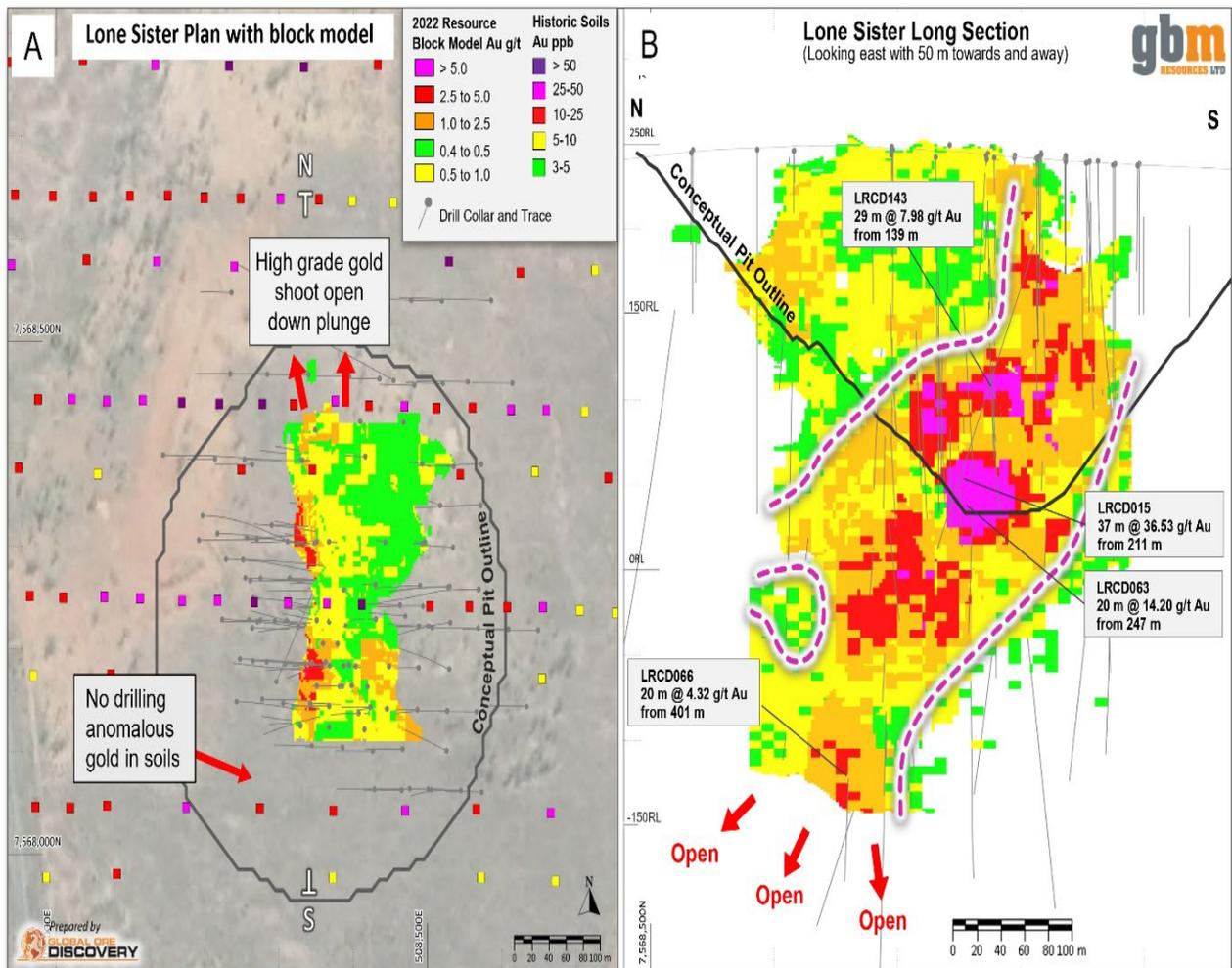
**Figure 7. A Plan (A) and cross-section (B) showing the recently released Lone Sister MRE block model. Note that high grades plunge to the north and remain open down plunge. This is a key target for GBM. Historic soil data and drill hole data are also shown.**
