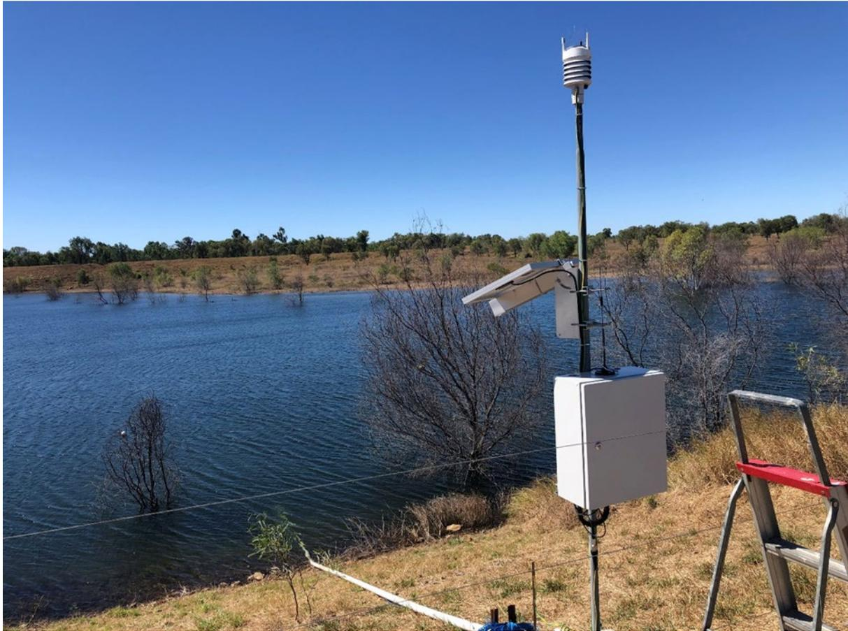
**Figure 34: New Weather Station to Assist in Environmental Monitoring Installed at Yandan.**
