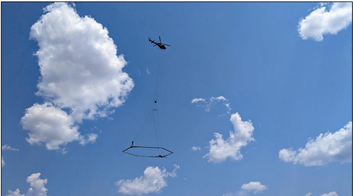
Figure 1 - Fenton Gold Project, SkyTEM AEM survey underway.
