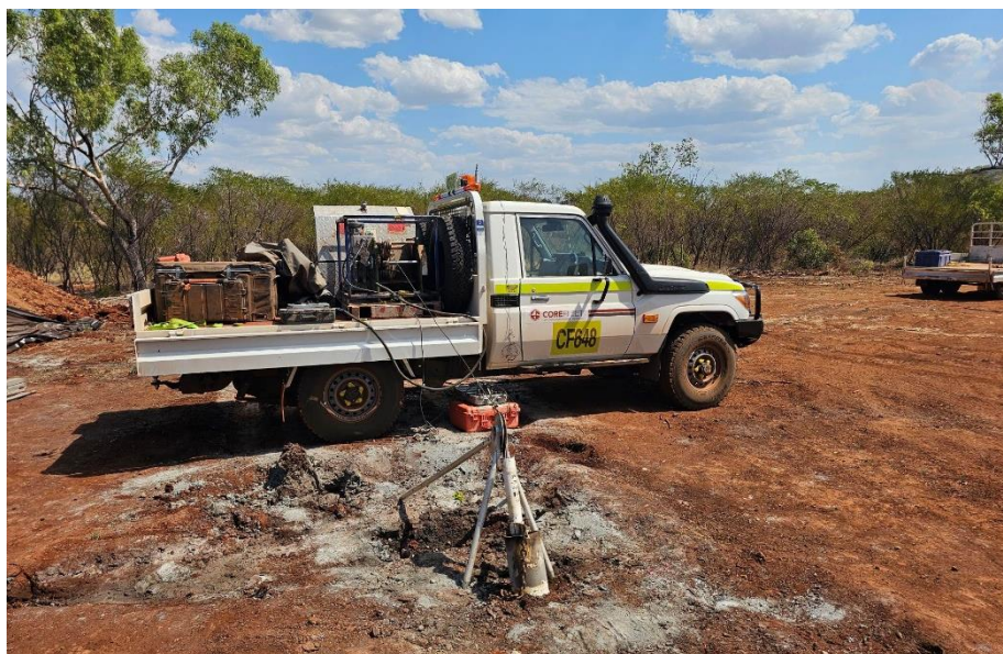
Figure 1. Downhole Electromagnetic Survey set up at BRDD001
