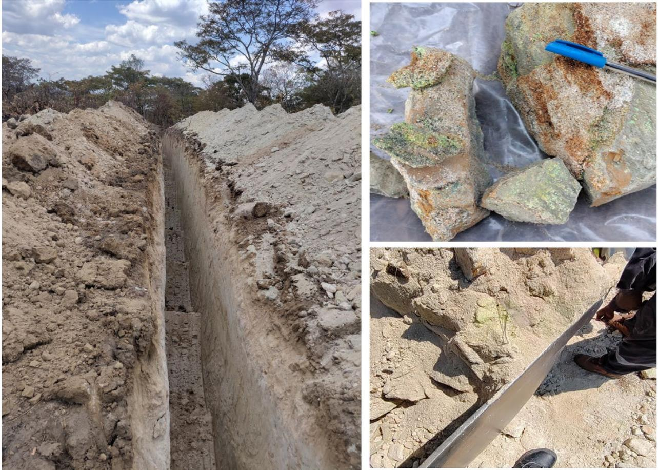
***Fig 3: Photographs of one the trenches and uranium mineralised (yellow) material***
