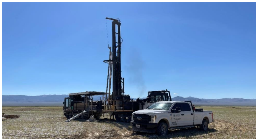
Figure 12: Sonic rig drilling at NBS Carvers
