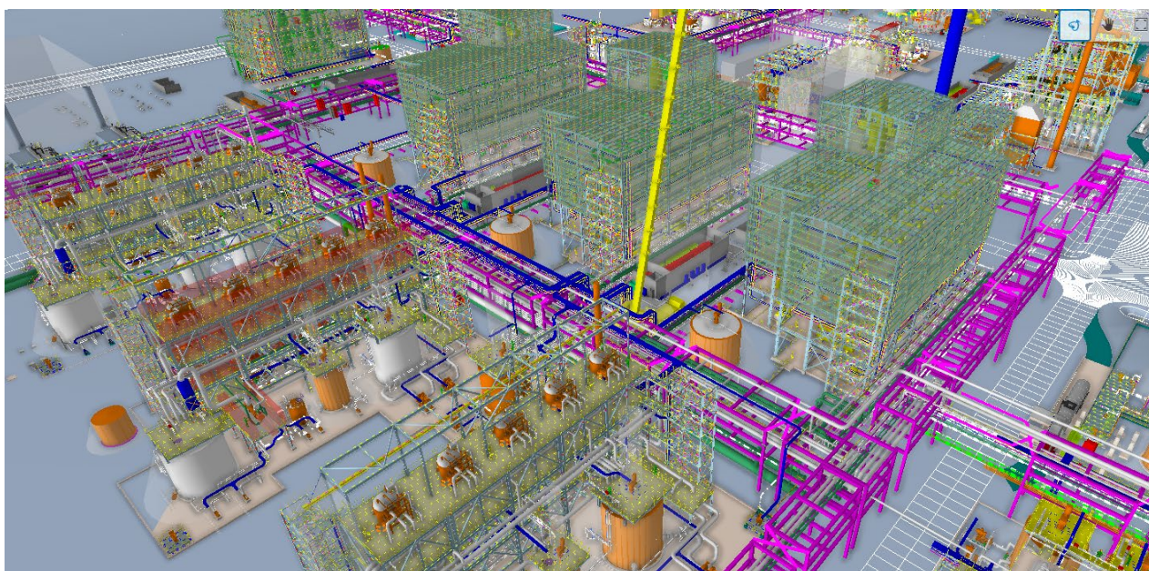
Figure: Pressure Iron Hydrolysis (KBR Package) which precipitates hematite and recycles nitric acid.
