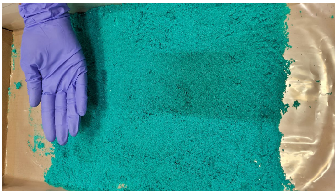
Figure: Nickel sulfate produced during pilot plant operation
