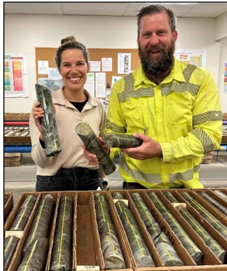
*Photos 2 and 3 – Chalcopyrite mineralisation in WTU-23-06 from 100m to 105.2m, within an 11.4m thick zone grading 2.29% Cu, 16.45g/t Ag and 0.14g/t Au. Bree Ivory (Corporate Affairs Manager) and Brian Paull (Director of Exploration) holding core from WTU-23-06.*
