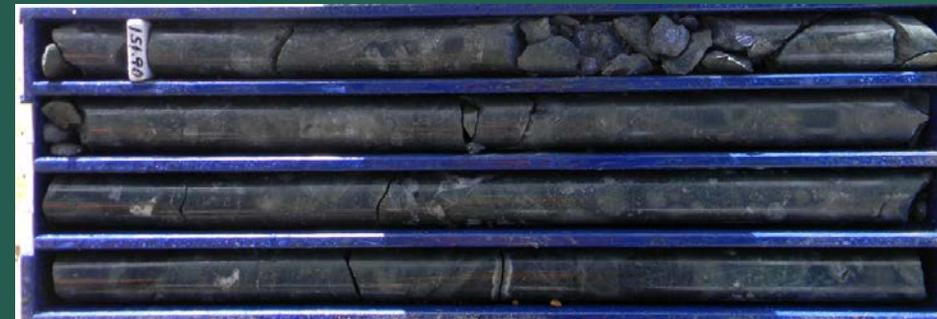
The core Sampled at point **B**) is a polymictic breccia clast supported, with strongly altered quartz-sericite (green)-chlorite angular hornfels and rounded felsic porphyritic clasts. Spaces filled with molibdenite cement, chalcopyrite, traces of bornite and granular silica .
