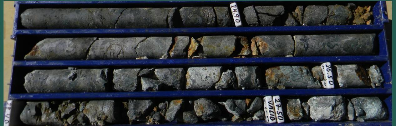
The core shown at Sample point D) demonstrates crackle breccia in hornfels, chalcopyrite, pyrite, traces of bornite in veins and disseminated molybdenite.
