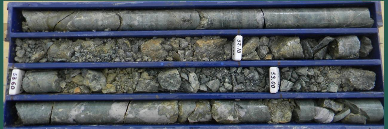
The core at Sample Point E) shows clast-supported breccia dominated by hornfels and sporadic fragments of felsic intrusive with porphyritic texture, filled with molybdenite and chalcopyrite and rock flour matrix.
