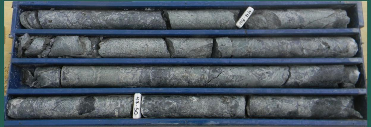
The core sampled at point F) shows Clast-supported breccia dominated by quartz monzonite equigranular intrusive and some fragments of hornfel, filled with molybdenite and chalcopyrite and rock flour matrix.
