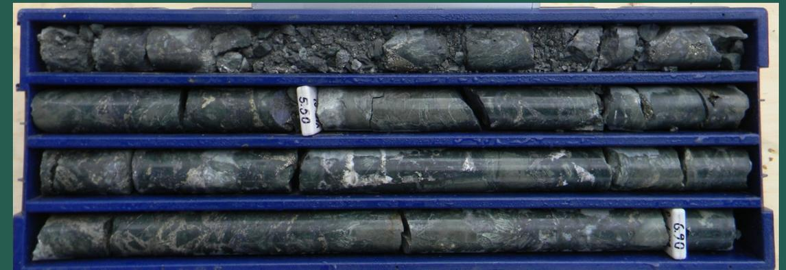
The core sampled at point **A**) is a monomictic breccia clast supported, with strongly altered quartz-sericite (green)-chlorite hornfels clasts. Spaces filled with chalcopyrite, molybdenite, pyrite and granular silica . Interval 4.5m-6.4m assays 1.9m @ 3.33%Cu, 0.598%Mo. (See a full list of assays in the ASX announcement of 4th May 2023)
