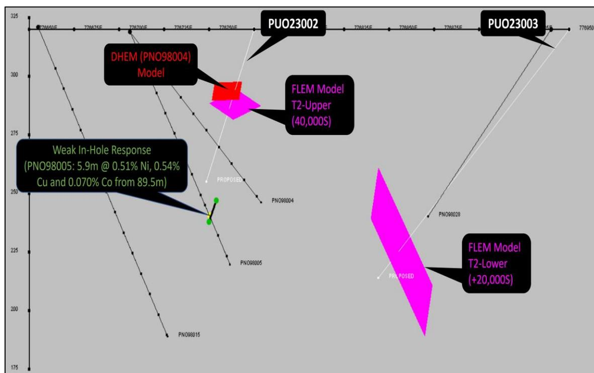
**Figure 1:** Sectional view showing the DHEM and FLEM conductor models for T2-Upper and T2-Lower recently drill tested by drillholes PUO23002 and PUO23003. NOTE: The intercept in green text is from historic drillhole PNO98005.
