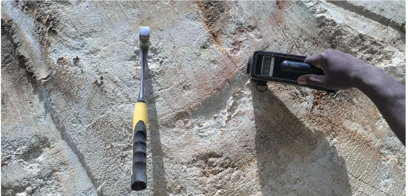
**Fig 2: New trench wall and scintillometer with >9,999 cps**
