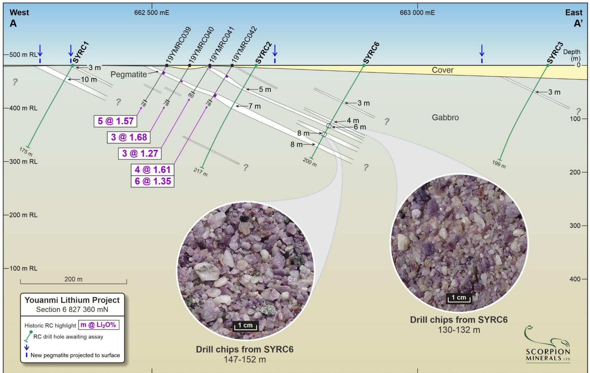
**Figure 2: Cross Sections 6 827 360 mN (A-A'), Showing new drilling and new pegmatite intercepts, and significant Li<sub>2</sub>O Drilling Results in Shallow East Dipping Stacked Pegmatites**
