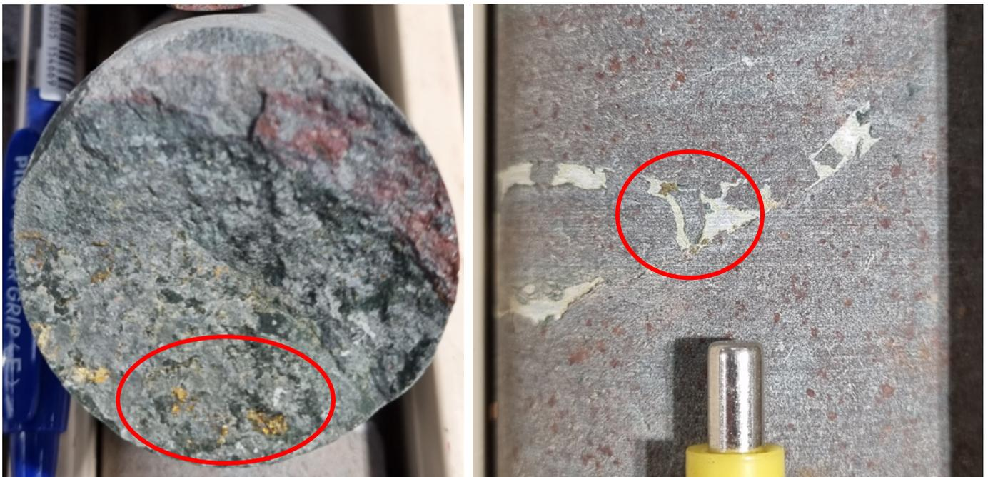
*Figure 1: Left –Chalcopyrite on fracture surface. Right – Tarnished chalcopyrite in carbonate filled fracture.*
