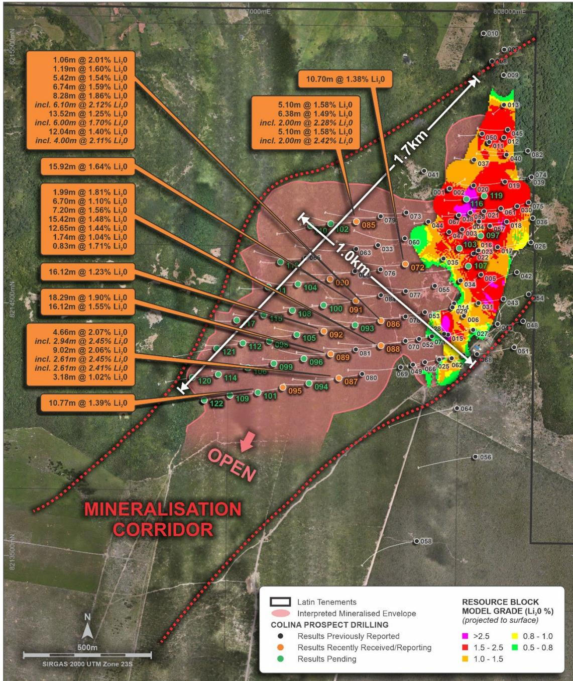
Figure 2: Colina Deposit drill collar plan highlighting potential MRE growth areas, including Colina West and Colina South
