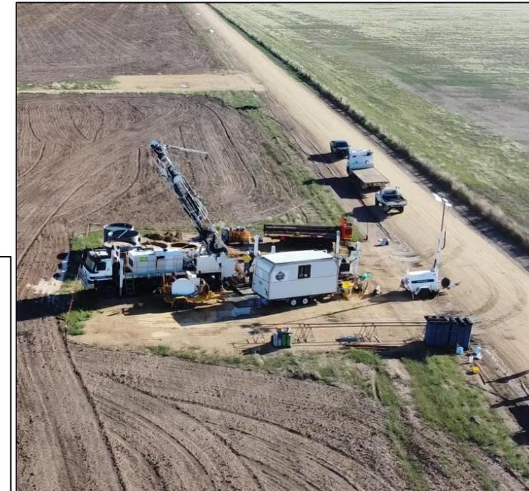
Drone photograph at Myall (looking northeast) showing the diamond drill rig set up on hole 23MYDD423, targeting a major expansion of the Corvette Prospect
