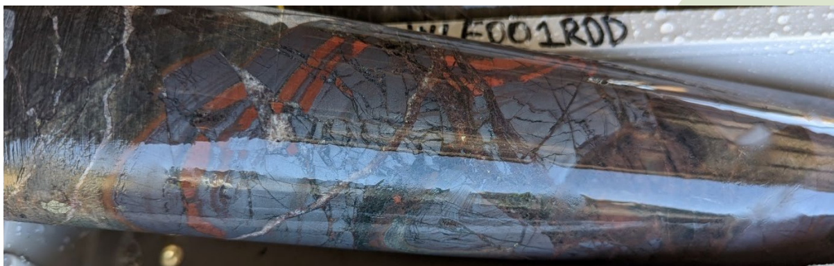
Figure 2. Ironstone that hosts 0.24% U_3O_8 mineralisation from 689.09 – 689.41m in drill-hole KNXLE001RDD.
