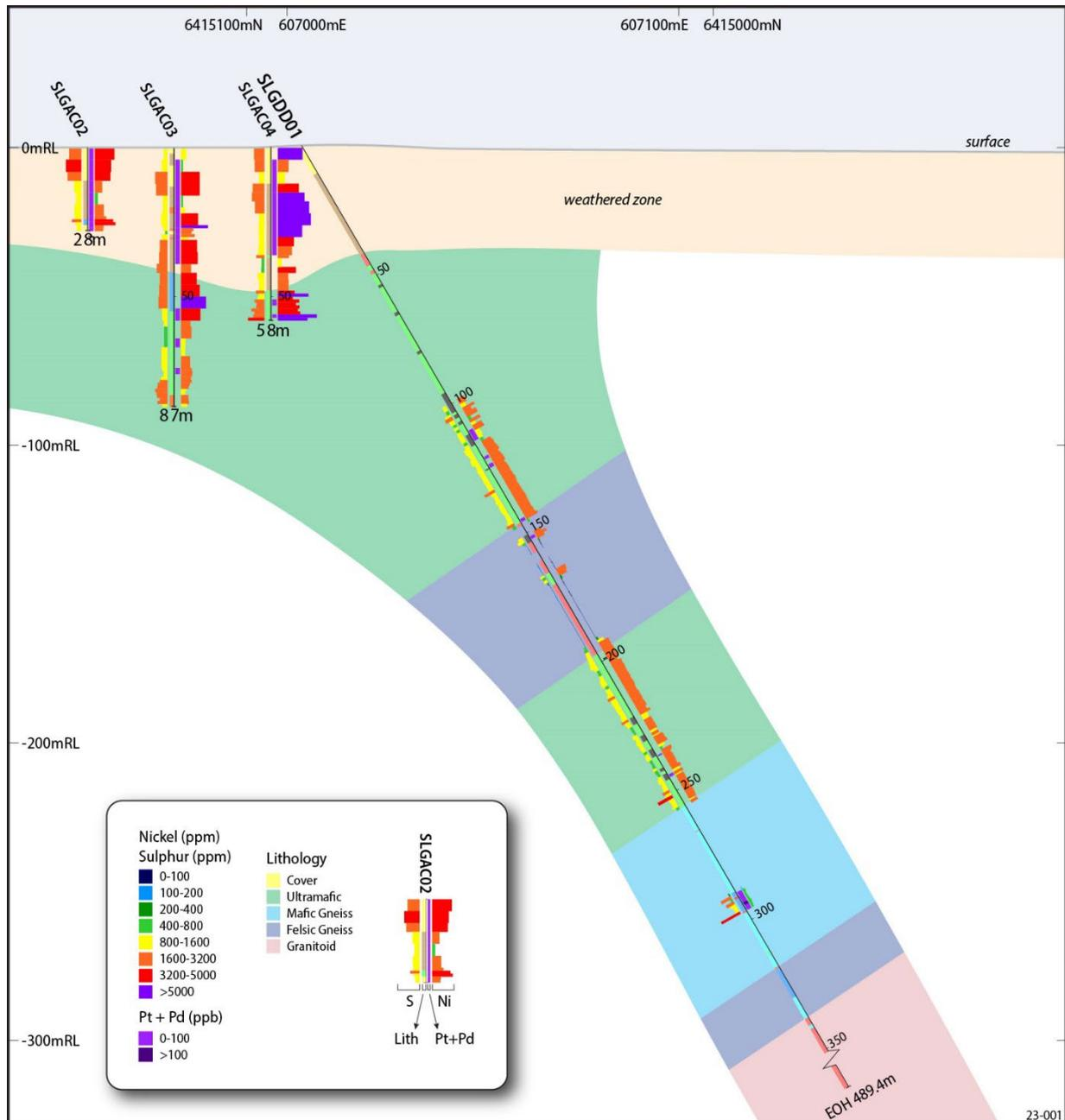
Figure 2: Cross-section of RC drill hole SLGD001 along with previous aircore drill holes SLGAC02, SLGAC03 and SLGAC04. Ni is displayed as a concentration based coloured histogram on the right hand side of the drill string, sulphur (S) on the left hand side of the drill string and Pt + Pd as a concentration based colour within the drill string.
