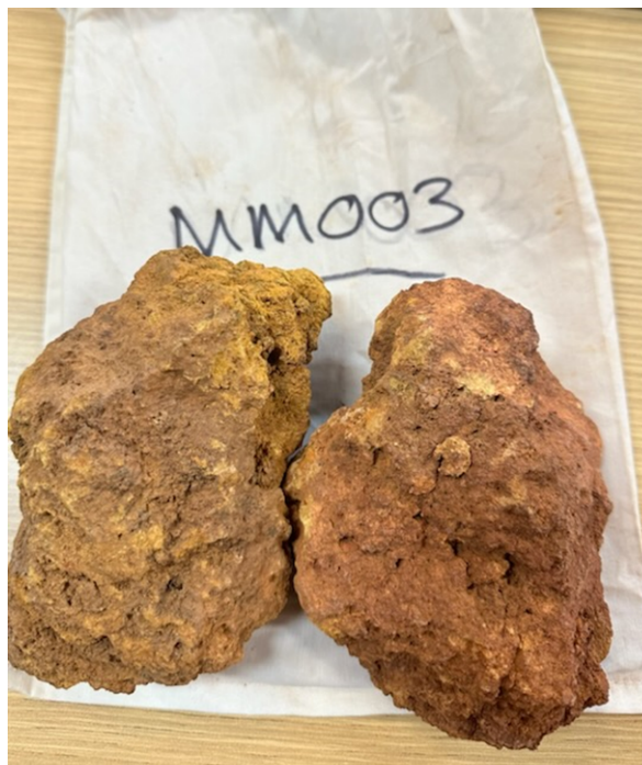
Figure 6: Rock Chip Sample MM003: 3.04 % Cu, 269 g/t Ag, 2.13 g/t Au, 0.71 % Zn and 9.25 % Pb
