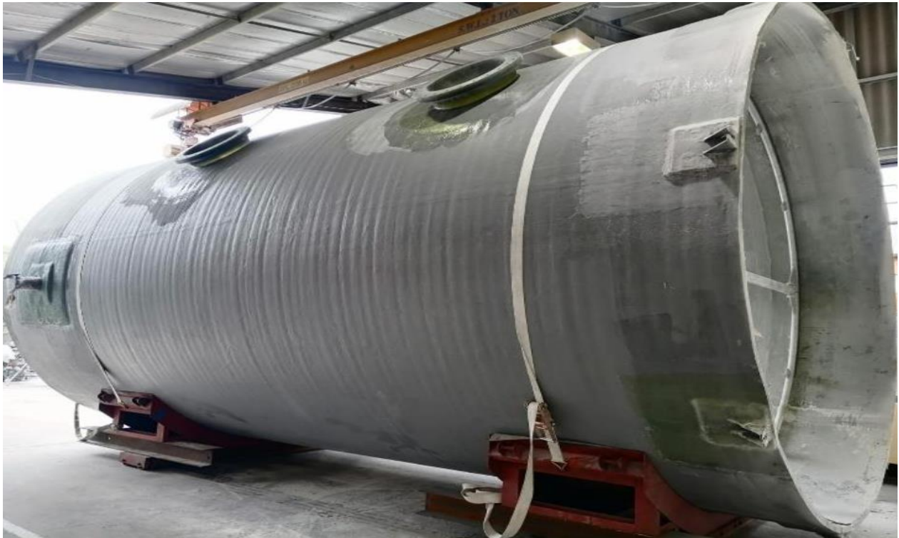
Image 1: First Ion Exchange cylinder winding complete.
