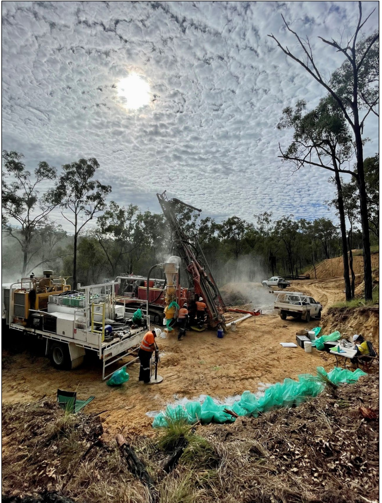
Figure 2: RC drilling at Triumph in April 2023.
