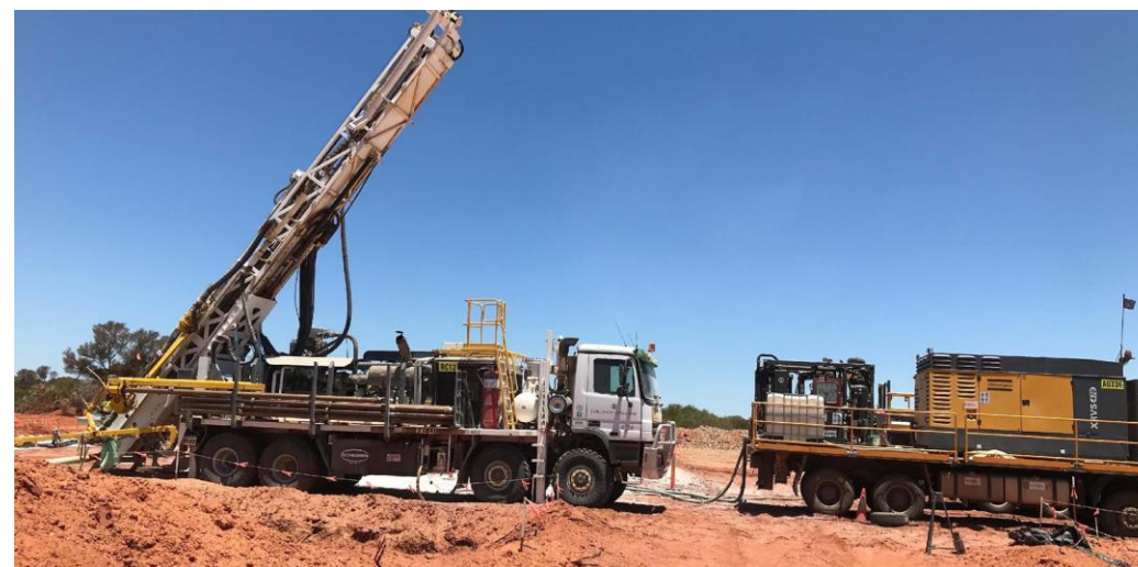
RC deep hole drilling to 450m+
