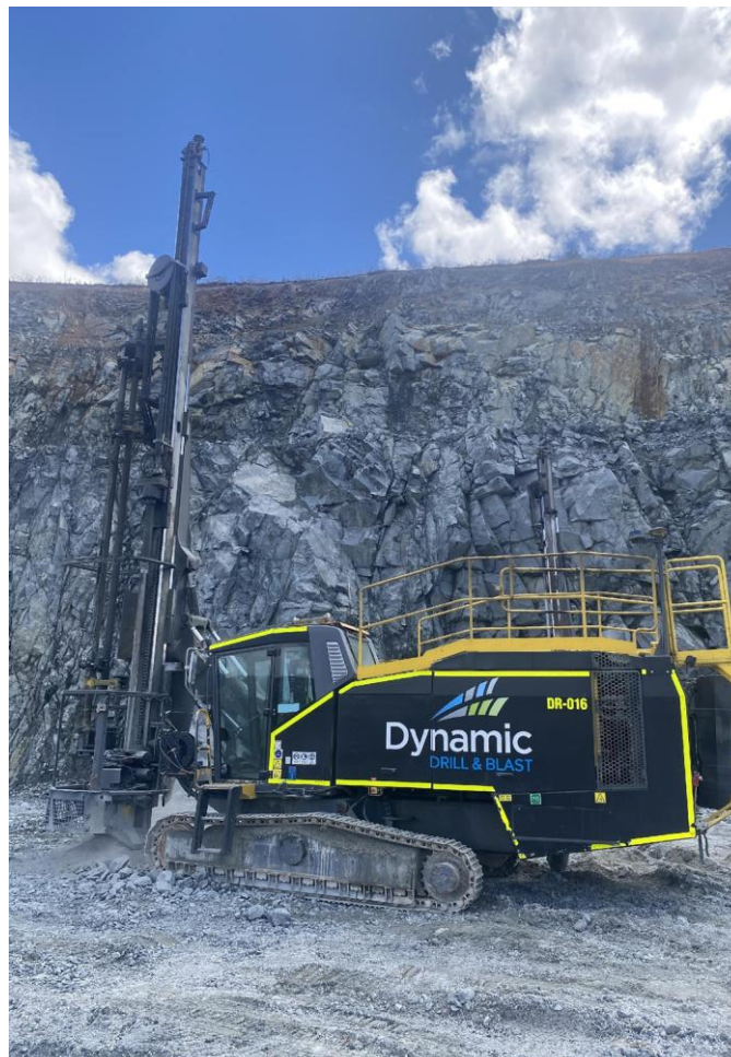
Epiroc D65 Down The Hole Hammer Drill Rig
