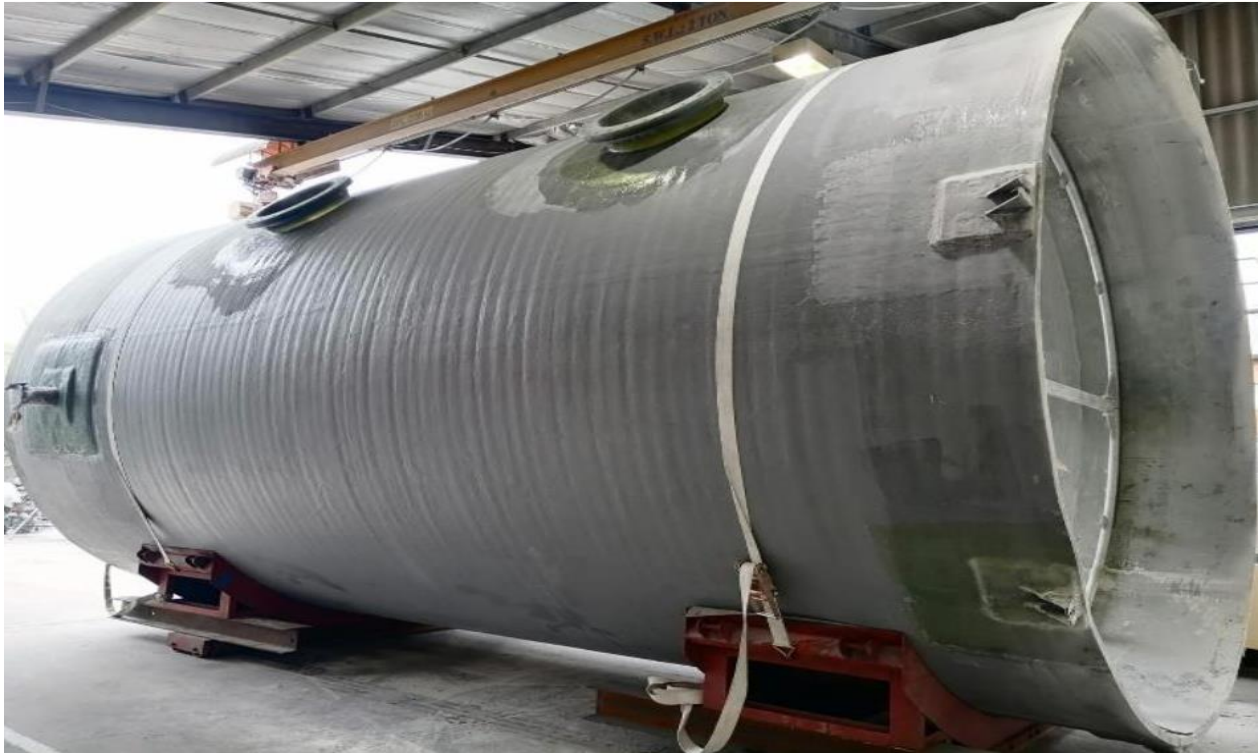
Image 1: First Ion Exchange cylinder winding complete
