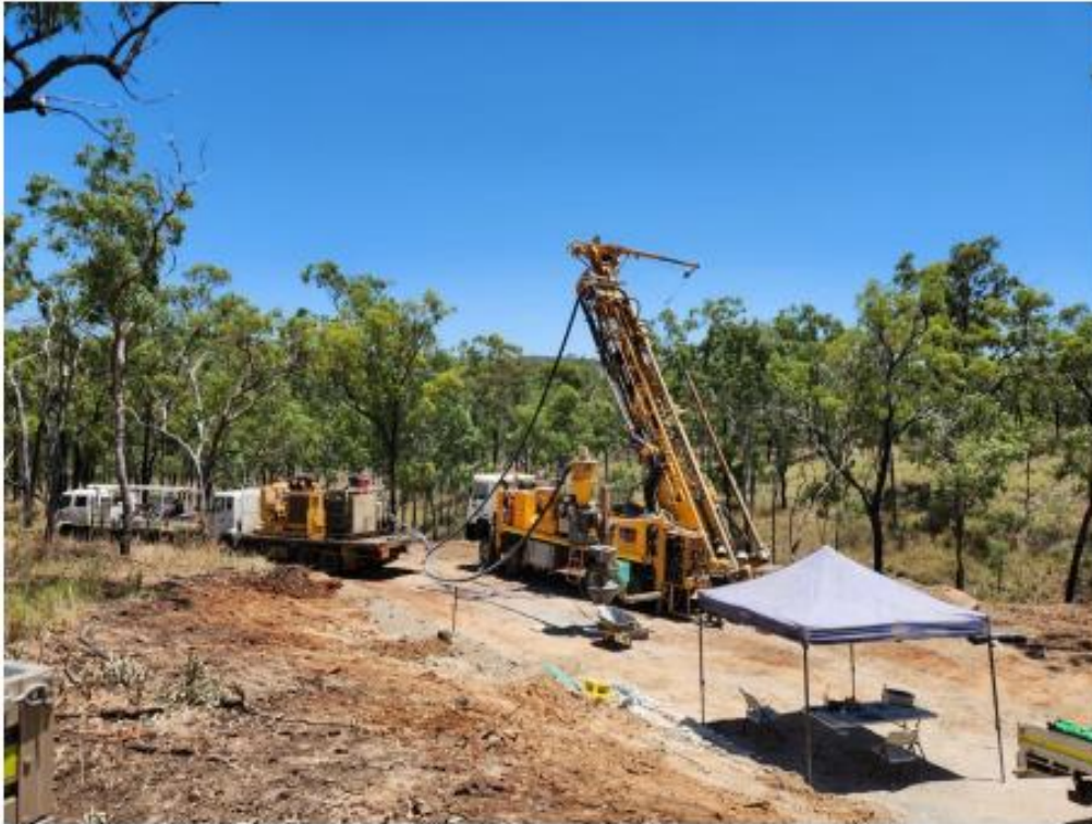
Figure 5 RC drill rig drilling at Douglas Creek
