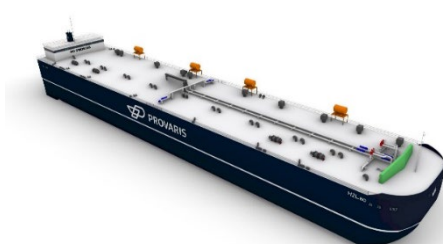
Figure 4: Illustration of the H2Leo 26,000m 3 compressed hydrogen floating storage integrated with H2Neo 430t carrier for loading or unloading.
