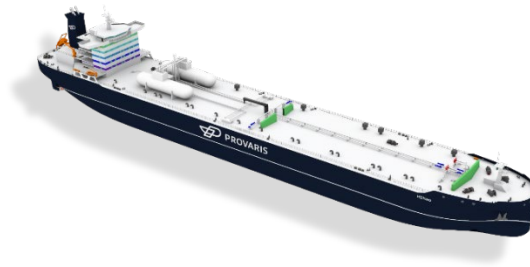
Figure 3: Illustration of the H2Neo 26,000m 3 compressed H2 carrier
