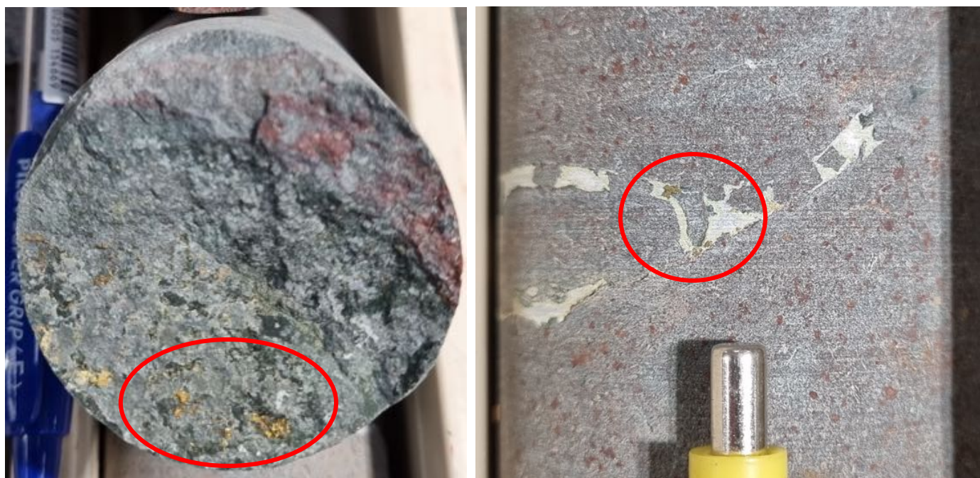
Figure 9: Left –Chalcopyrite on fracture surface. Right – Tarnished chalcopyrite in carbonate filled fracture. Core from Sample ID 610027
