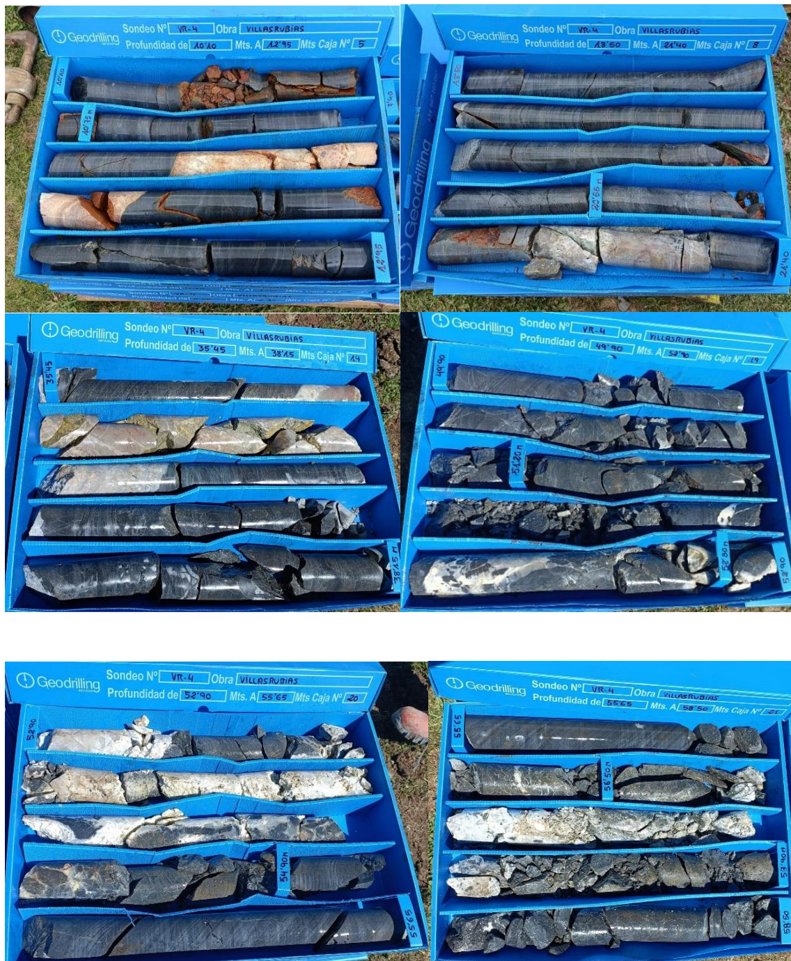
Different pegmatite bodies and dykes intercepted by well VR-4.
