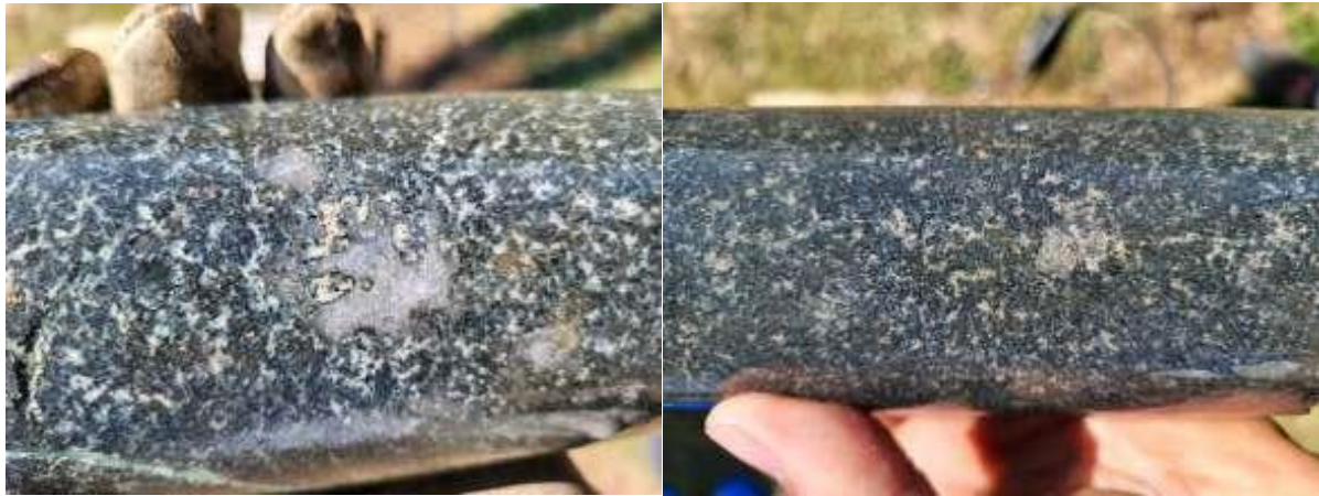
Picture of cores of probable mineralized gabbro intercepted by VR-1 and VR-3 over magnetic anomaly.
