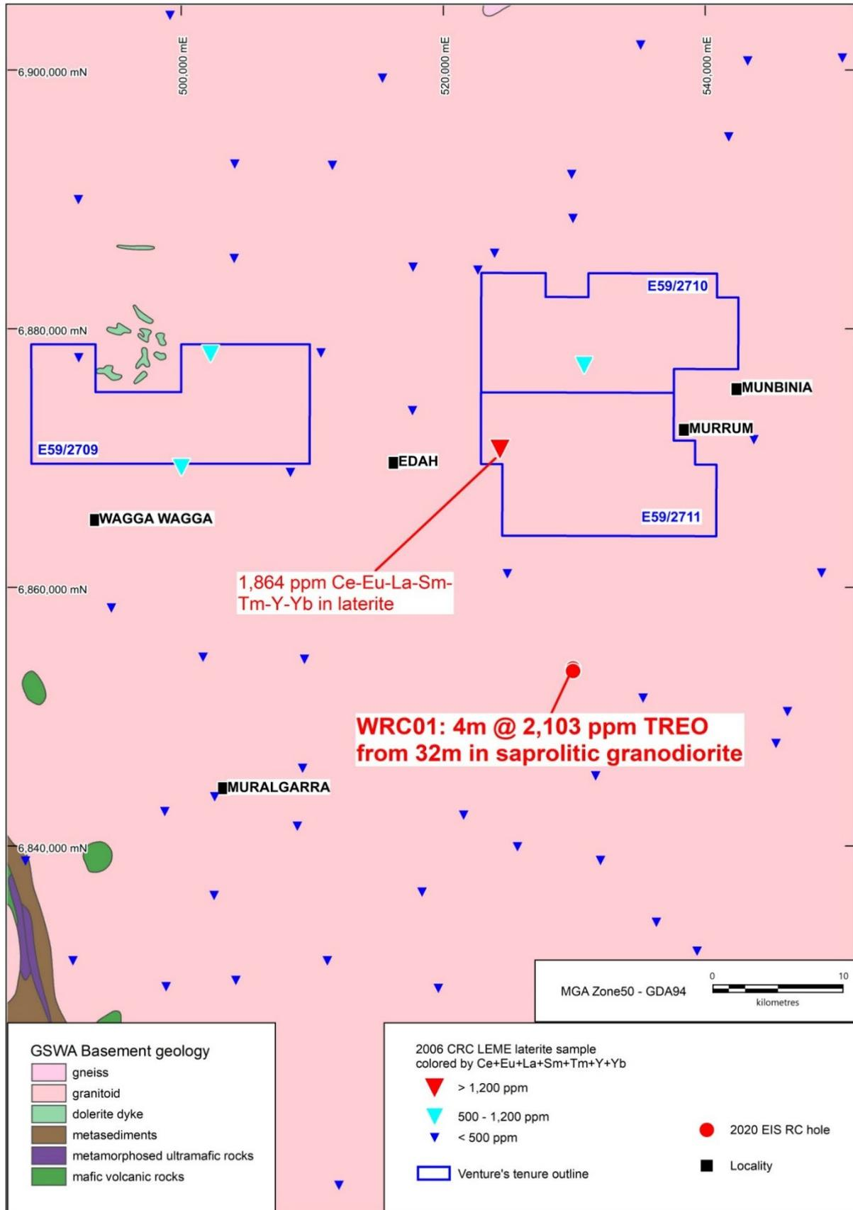
Figure 6 | Bandy Project: Geology Map showing REE laterite geochemical sample results.
