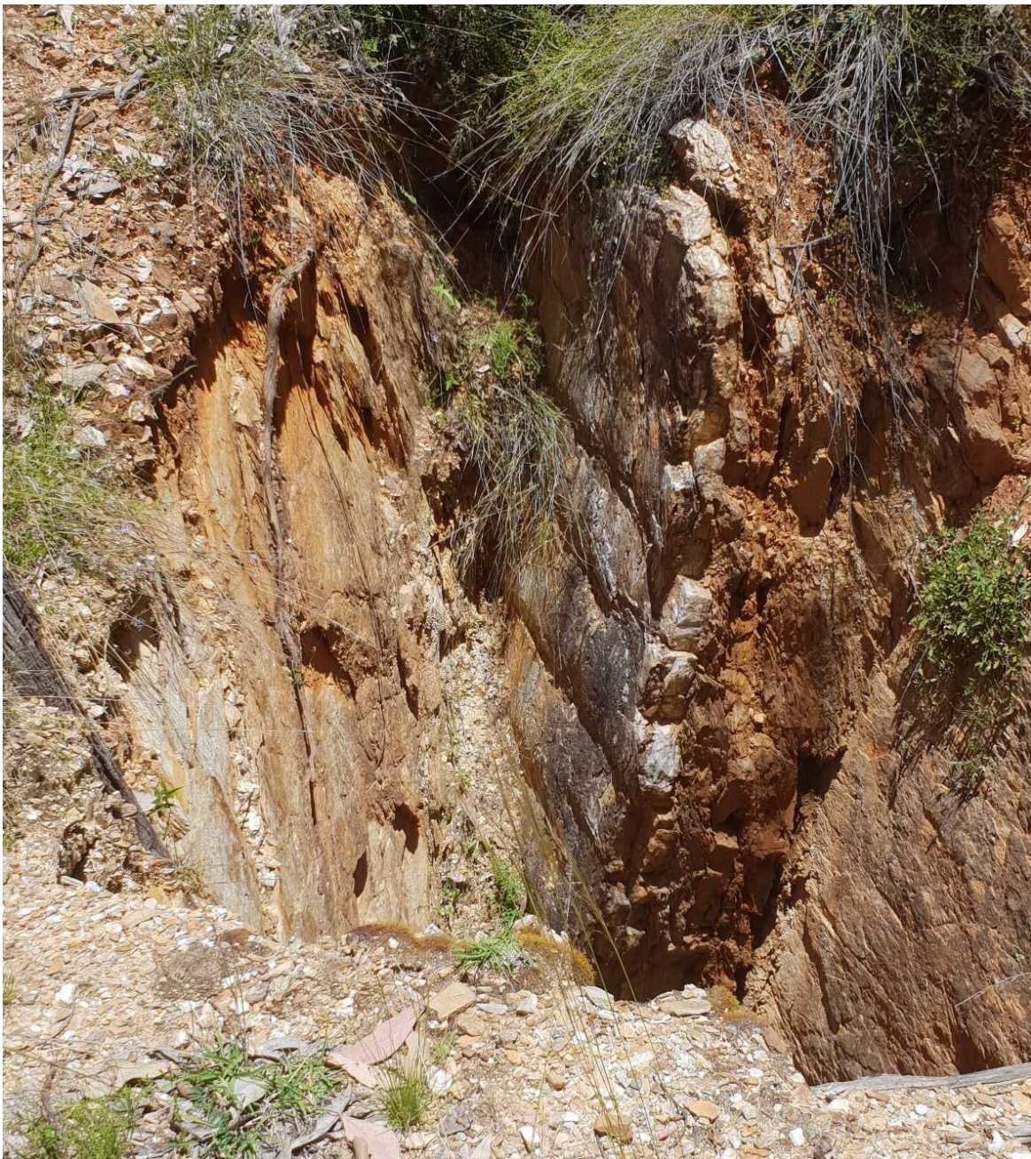
Image 1: Tuckers Hill Project, workings on east dipping high-grade gold bearing quartz lodes
