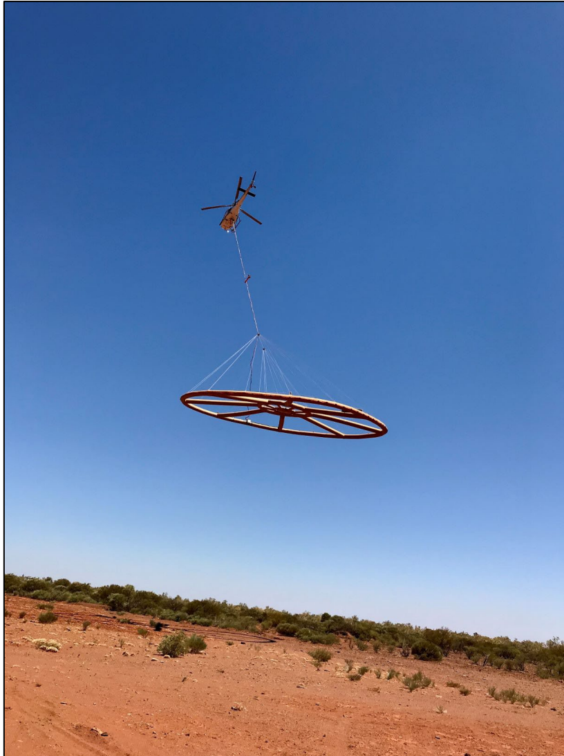
Figure 3: NRG helicopter based AEM survey.
