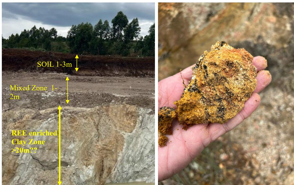
**Figure 3. a)** From Togni SA refractory clay mining pit at Capo do Mel (CDM) Project highlighting the thin soil horizon (approx. 1m this area) underlain by a mixed clay soil zone 1-2m thick and then a mineralised clay zone enriched in REE.
