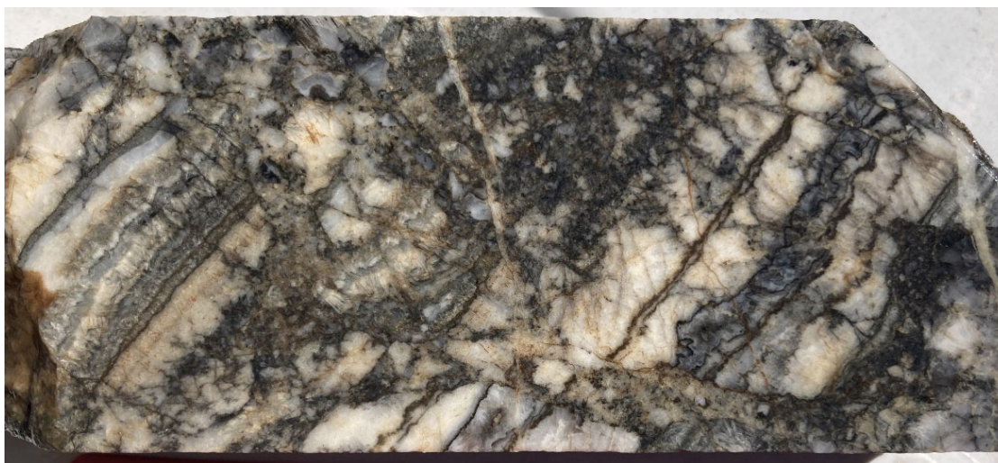
Figure 3. A photograph of an East Hill high-grade vein from 350.5 m in YAN010 that assayed at 145 g/t Au (Refer ASX:GBZ release 23 December 2020). Note the colloform, crustiform, and bladed textures.
