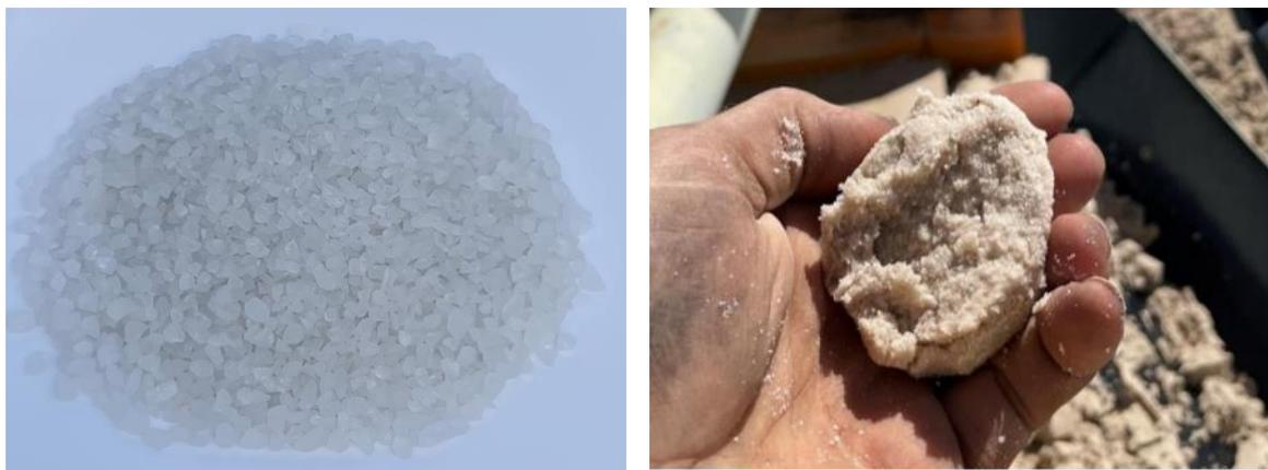
*Plate 2: Left: -4.0mm, + 2.0mm crushed HPQ from Karatha. Right: Stockyard HPSS product sent to China for beneficiation testwork.*
