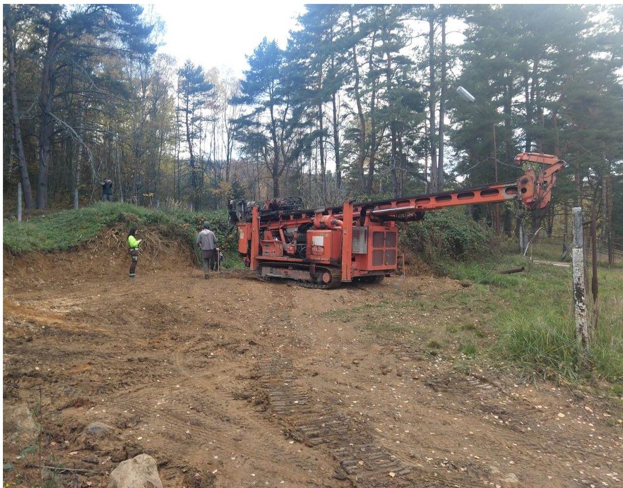
Figure 10: Diamond drill rig set up at the first target area, site preparation completed, location of drill hole SSD-01
