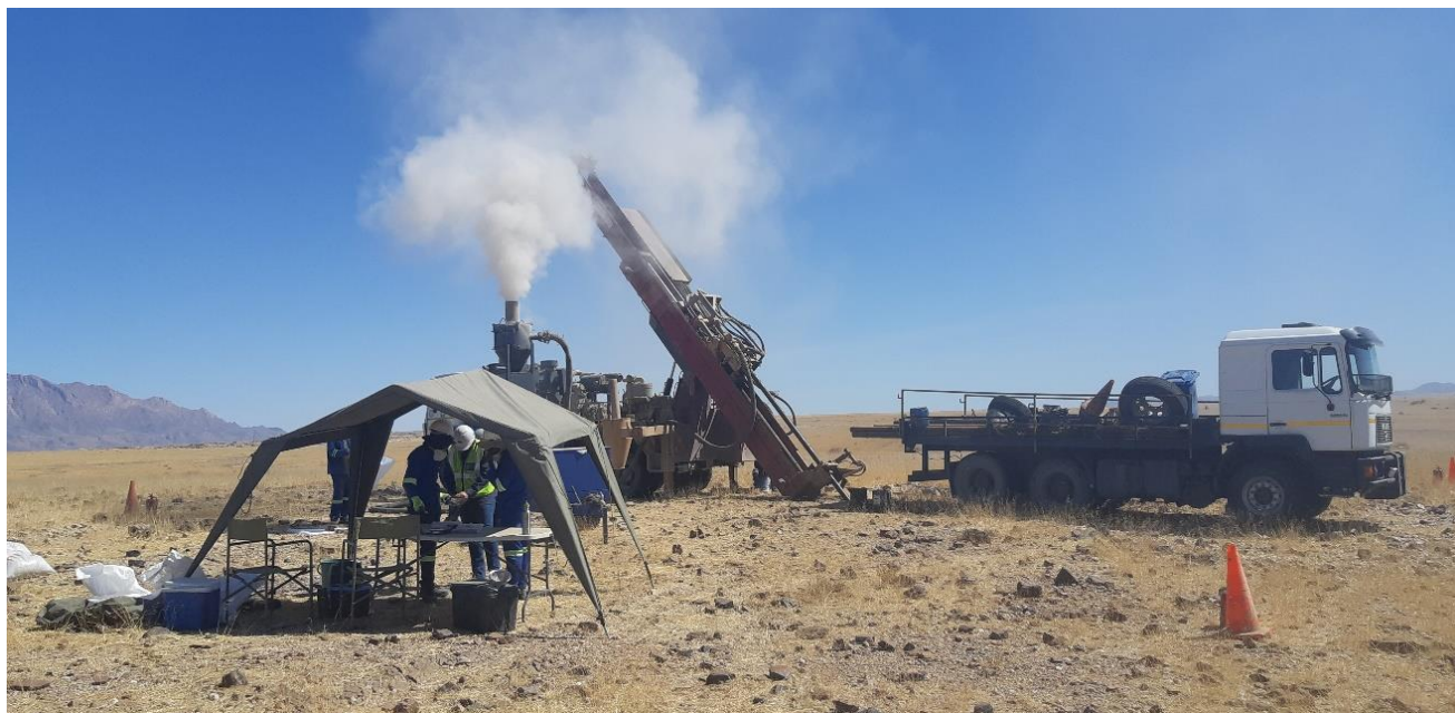
Figure 7: RC drill rig in operation at Area 1 within EPL 8535
