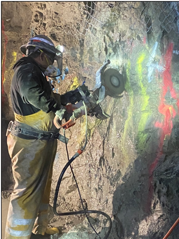
Photos 1 and 2 – Channel sampling of underground walls showing exposed mineralisation. Note sample width is approximately 2.5cm.
