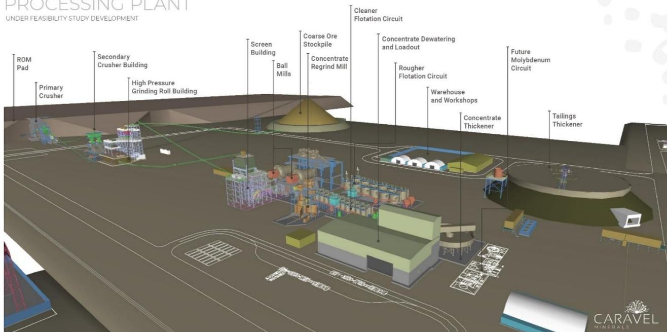
Figure 1: Proposed layout for the PFS optimised processing plant at the Caravel Copper Project
