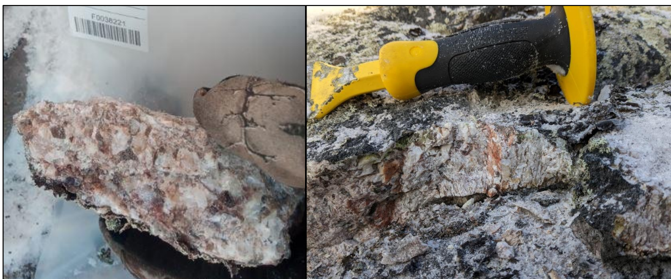
Figure 1: Selected photos of pegmatites from Zone 2. Left - Coarse grained pegmatite outcrop showing graphic texture. Right - Pegmatite sample F0038221 with coarse grained plagioclase + potassium feldspars, quartz, and muscovite (8.71 ppm Ta)
