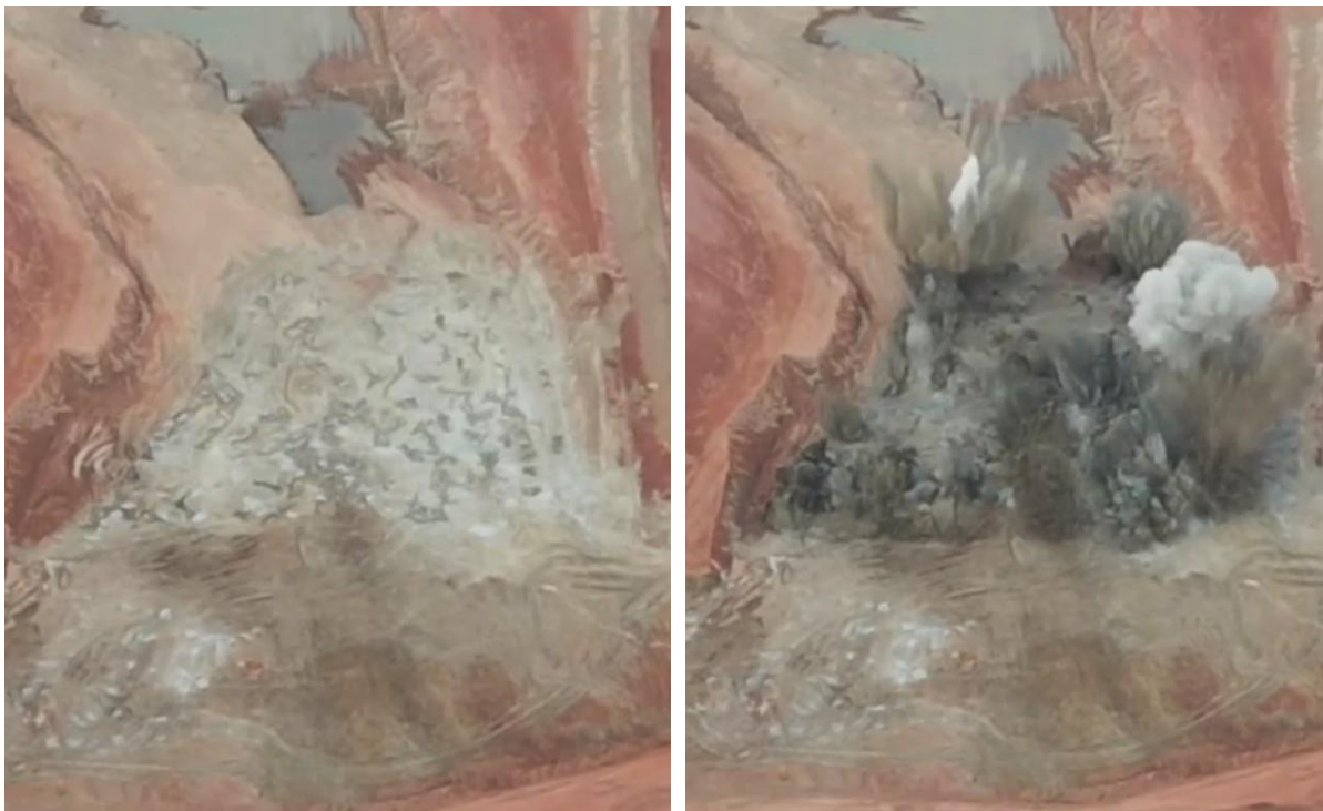
Figure 2: Images from the first blast of fresh rock at Abujar
