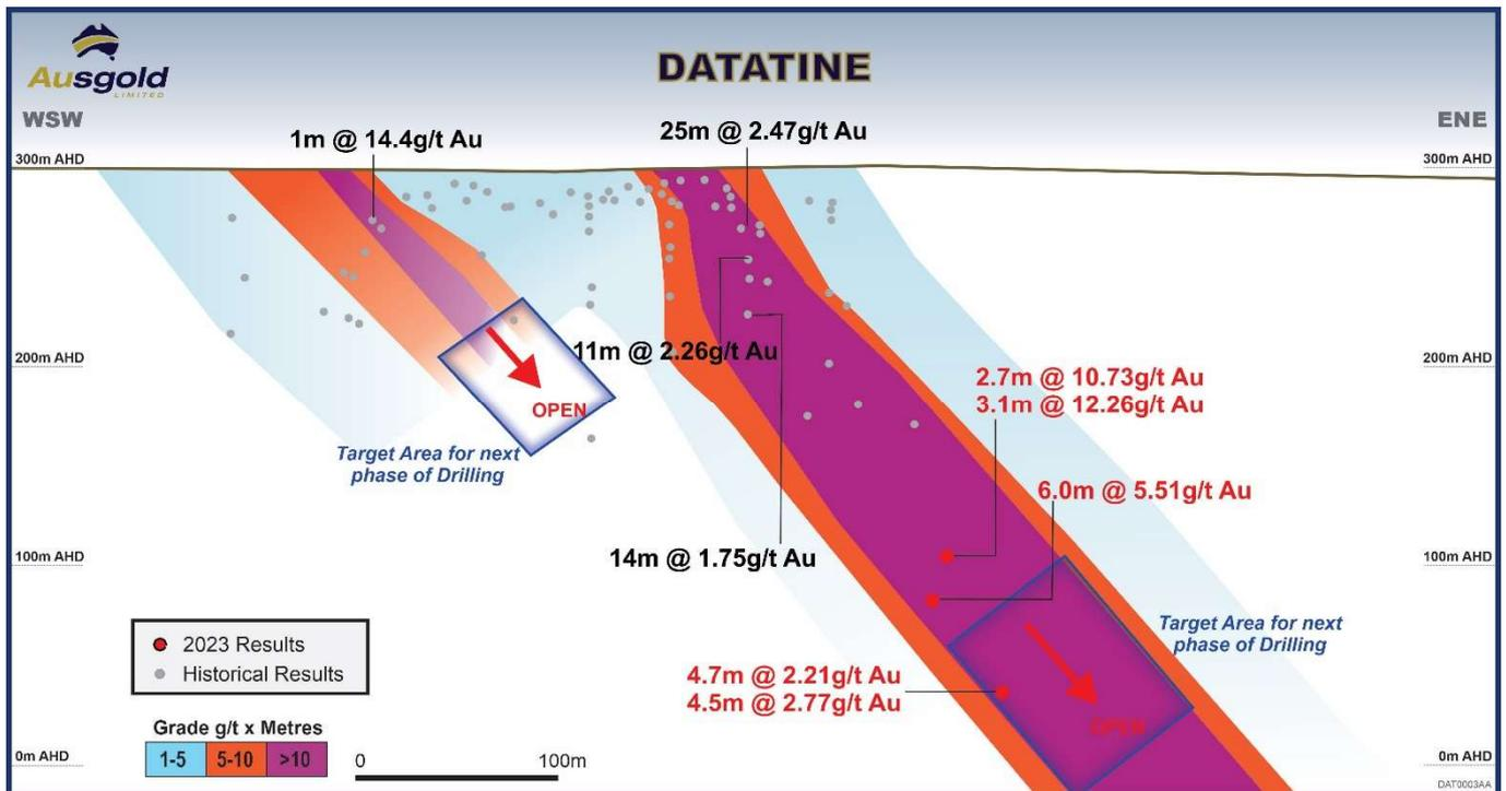
**Figure 7– Long -section of Datatine looking NNW**
