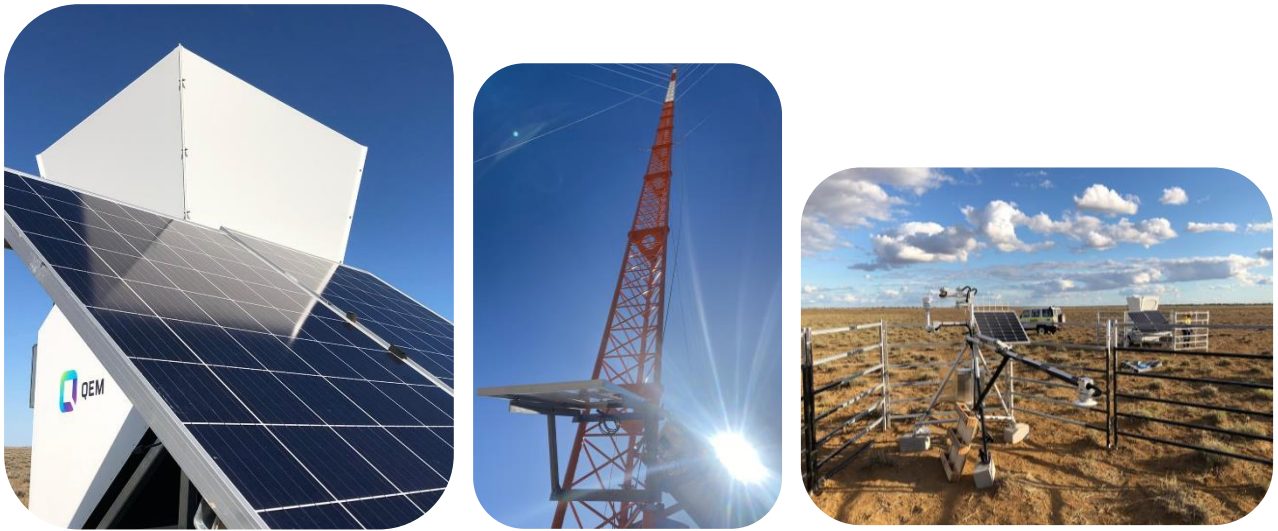
Images: QEM's solar and wind monitoring equipment onsite at Julia Creek
