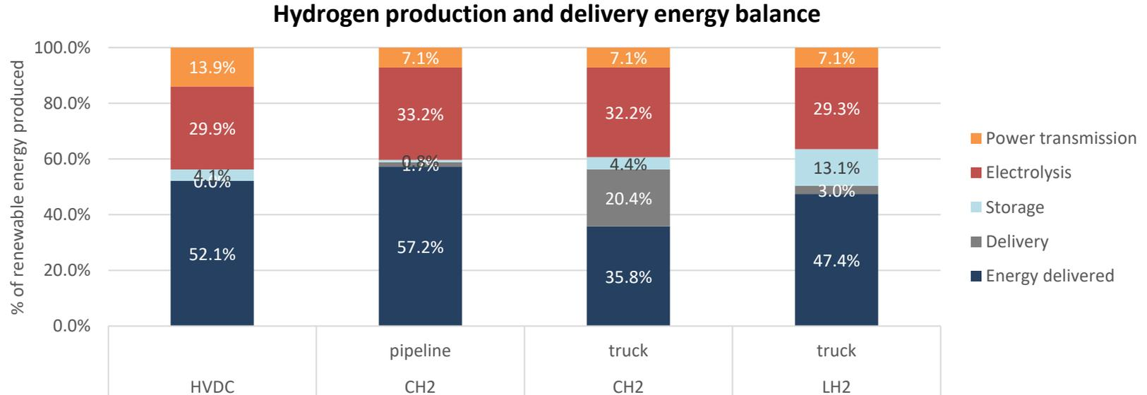
Option 1: Renewable power transmitted 500 km via high voltage direct current prior to green hydrogen production at customer site. Hydrogen compressed and stored at 35 MPa at customer site.
